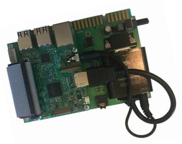
RpiCADE is the solution to a whole slew of issues that retro video gamers have. It is an extra board set that you hook up to your Raspberry Pi computer. It allows you to do the equivalent of RetroPie, which so many people are using to build handheld computers and retro mini-machines, but on your arcade cabinet. Supporting all the major emulators, it can also be the solution if you have an arcade game's boardset that went out on you.
